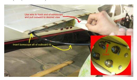
Inspection should cover the areas surrounding the four attachment nuts and extending upward and downward to the elevator skins and at least 1" inboard and outboard from the nuts. If suspect areas are noted, proceed to Step 4.
