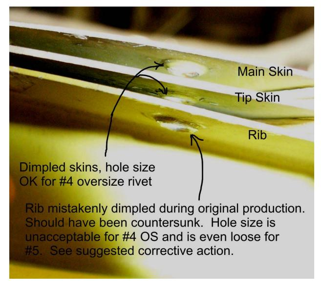
The Gulfstream repair corrective action procedures allow for recovery of cracked or compromised dimples by dimpling an AN960 (-6 in this case) and using it as a backup. DER prefers using a CSK washer, see picture, because of the larger footprint, and recommends structural adhesive in the buildup to fill the gaps caused
